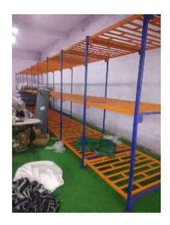
small fabric dimension heavy duty fabric storage rack is dimension size 4 fit x 4 fit x8 fit rack material heavy 50 mm x 25 mm ms sq. pipe powder coating size 4 fit x 8 fit frame size and ms sq. pipe 50 mm x 25 mm & 25mm x 25 mm shelf size (L 46"x W 46") per one rack 3 pcs shelf loading capacity one rack 1500 kg you are not provide single pieces rack your running pcs provide maximum 5 piece rack one set loading capacity valid one rack 1500 kg all racking system foldable
