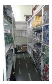
Accessories storage rack system and finish good storage rack dimension (2 fit W 4 fit L 7fit H) material description ms sq. pipe powder coating size 30 mm x 30 mm and pre laminated particle board wooden margin with palice all rack foldable& individual one rack capacity 500 kg all racking system foldable
